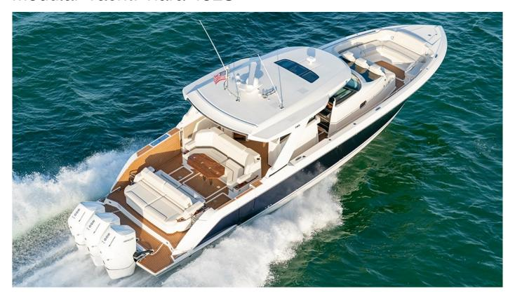
In the last decade, foldout and side-deck transoms, along with other modular designs, have become all the rage for boats over 40 feet. But US builder Tiara decided to approach the trend from an entirely different angle: For its <u>new 48 LS</u>, which has a fold-down side that opens up the rear quarter, the designers also created a less-is-more seating arrangement that pivots 180 degrees, while also sliding fore and aft, to offer multiple layouts.
